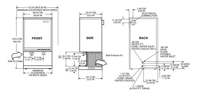
INSTALLATION NOTE: Allow 6" minimum space at sides and back for ventilation and utility connections.
