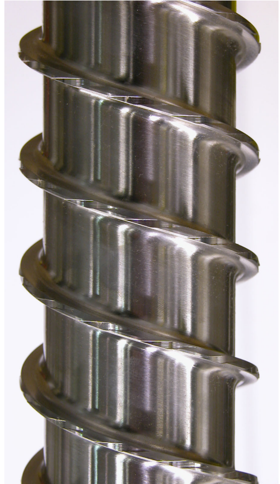
Example of a Clean Auger
