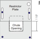
lce dispenser agitation setting should be set to .5 seconds. Set Motor Off time to 3 hours (see Figure F).
