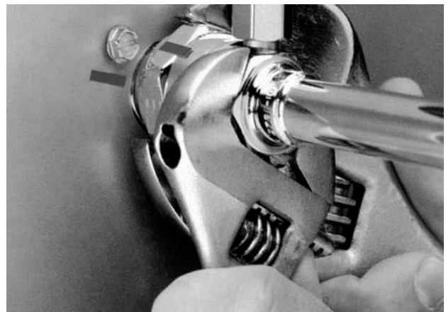
Rotate Swivel Nut ¼ Turn More
