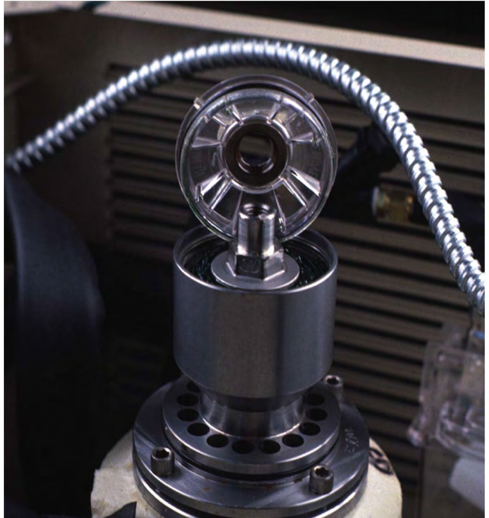
Bearing Cover removed (left hand threads)
